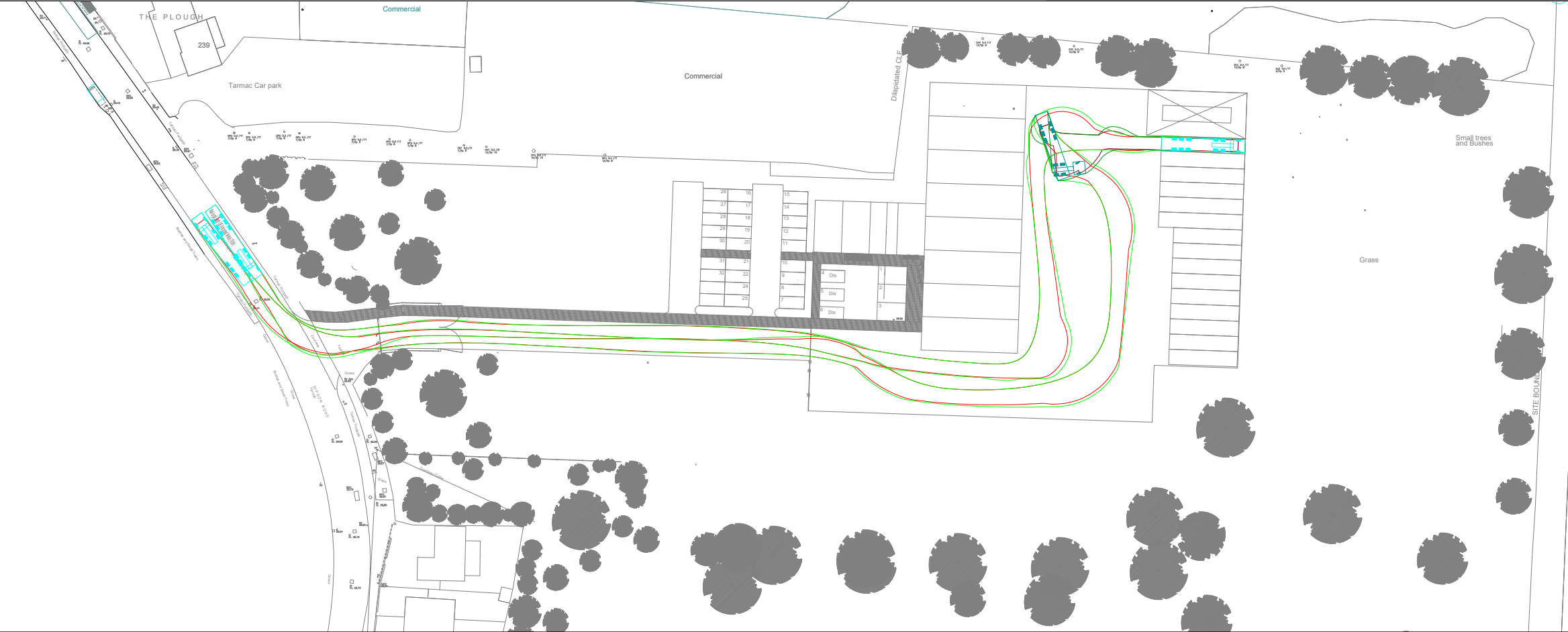
OVERALL SITE LAYOUT 16.5M ARTICULATED VEHICLE TRACKING (1:1000)
