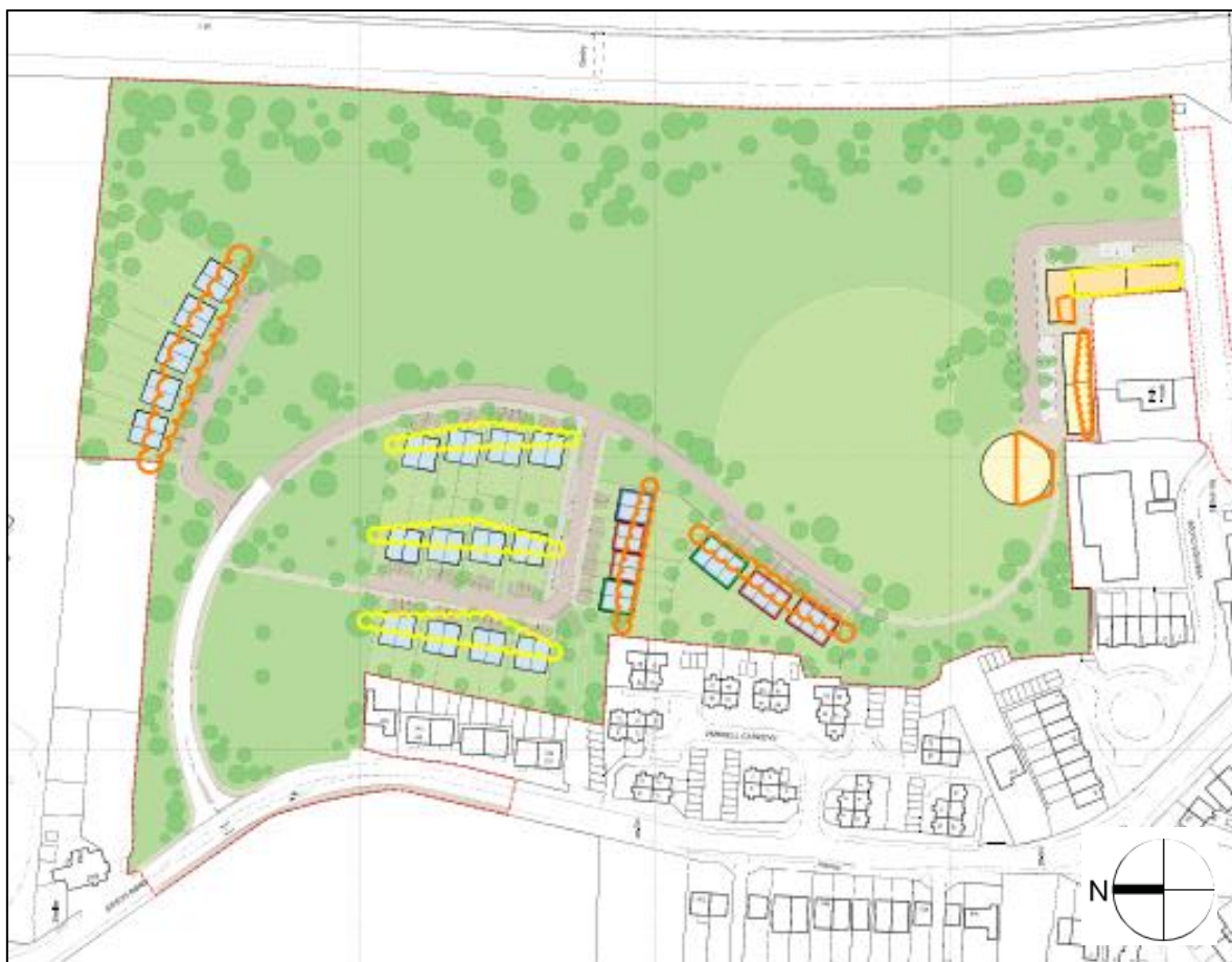
Figure 9: Annotated site plan showing very good locations for solar energy generation (orange) and acceptable locations (Yellow).
