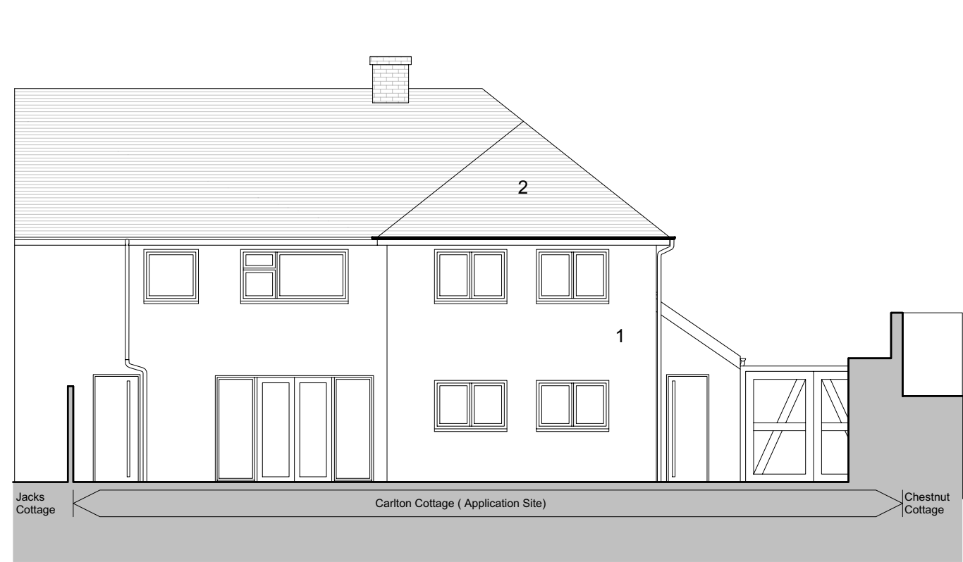
10 Proposed Elevation AA ( Rear) Scale: 1:100
