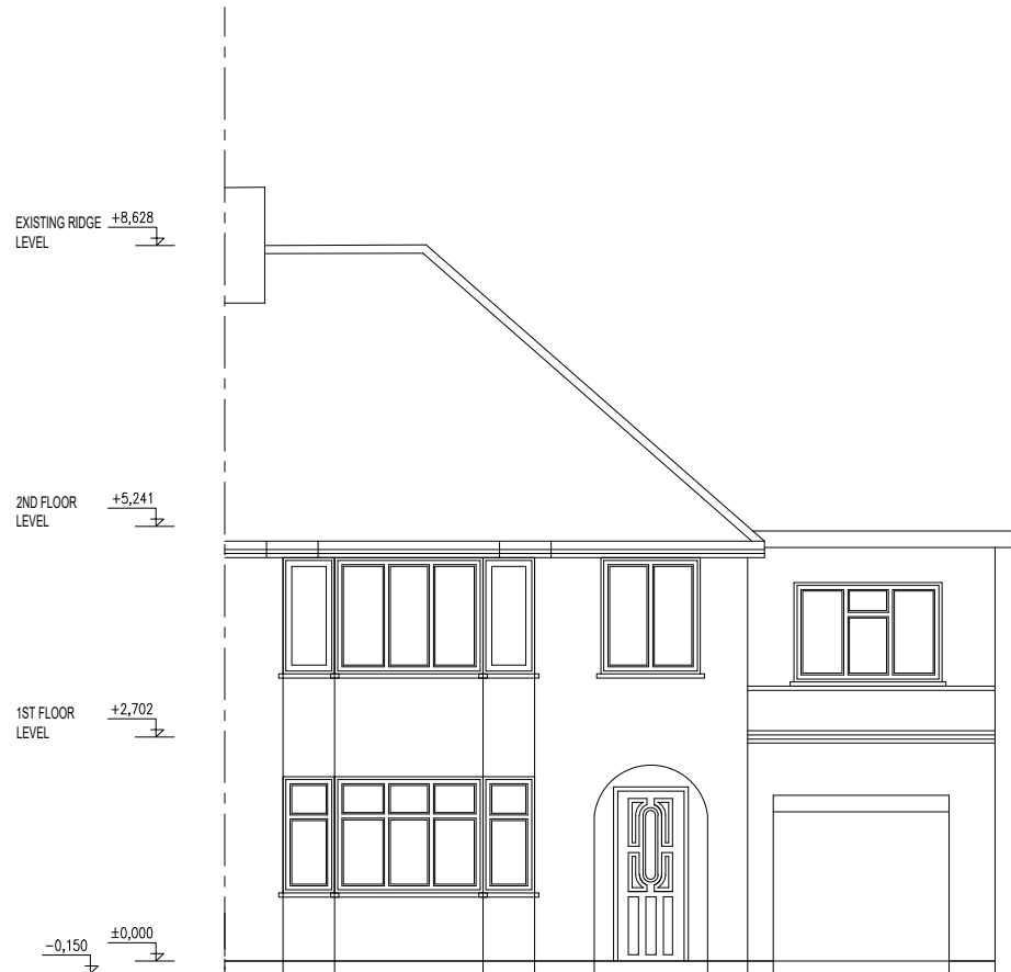
EXISTING FRONT ELEVATION 1:100
