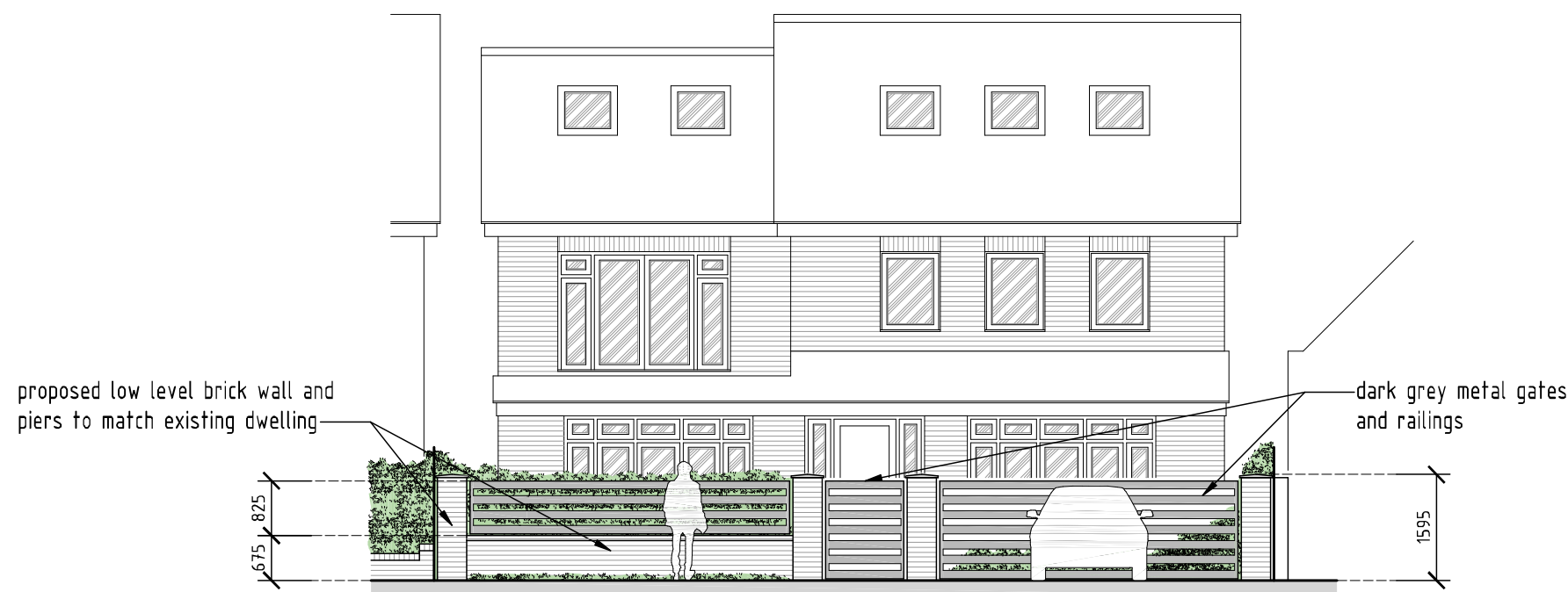
PROPOSED GATE, WALL AND RAILING DETAIL SCALE 1:100
