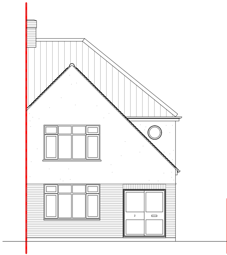
1 Existing Front Elevation 1:100
