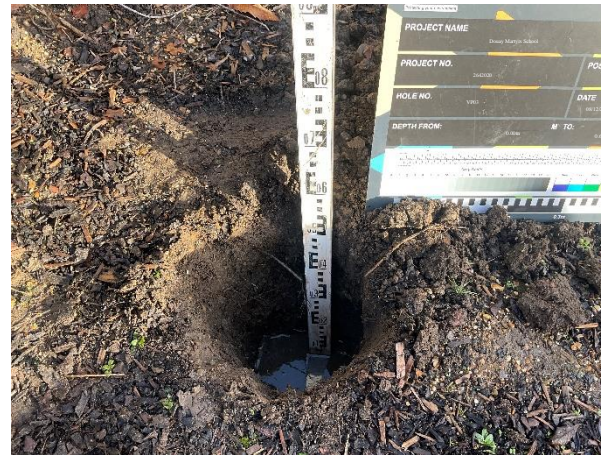
Photo 6: View of VP03 (water encountered at base of excavation, base of excavation observed prior to groundwater)
