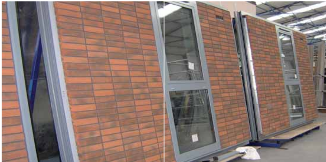
Parry Bowen Ltd - Hurst Street, Liverpool, unitised aluminium framed panels manufactured to \pm 1 mm tolerance
