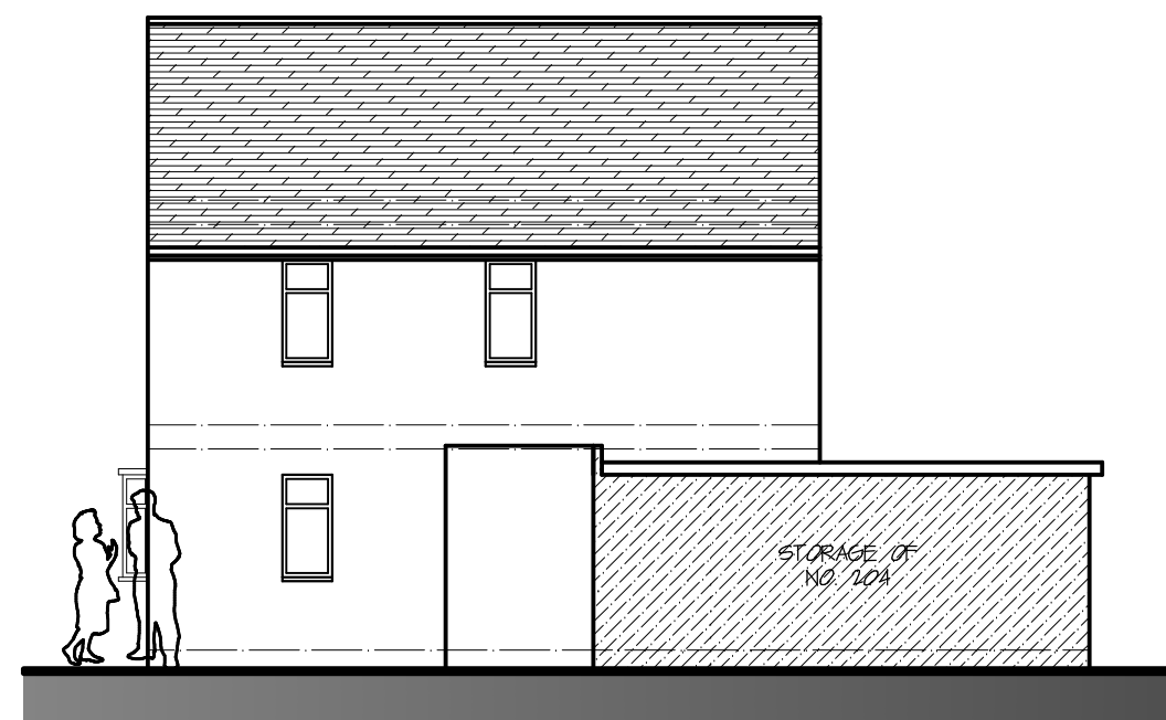
EXISTING OTHER SIDE ELEVATION
