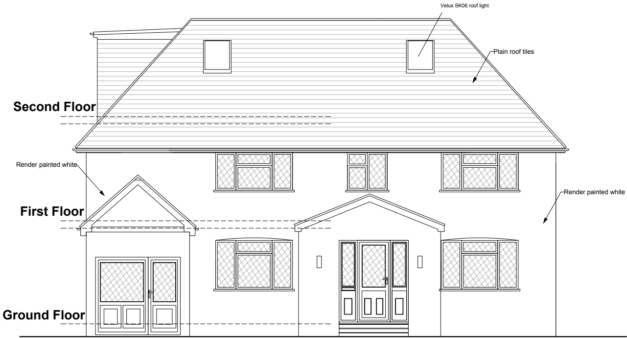
As-Built Front Elevation
