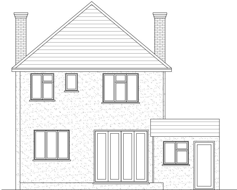
Existing Rear Elevation Scale 1:100
