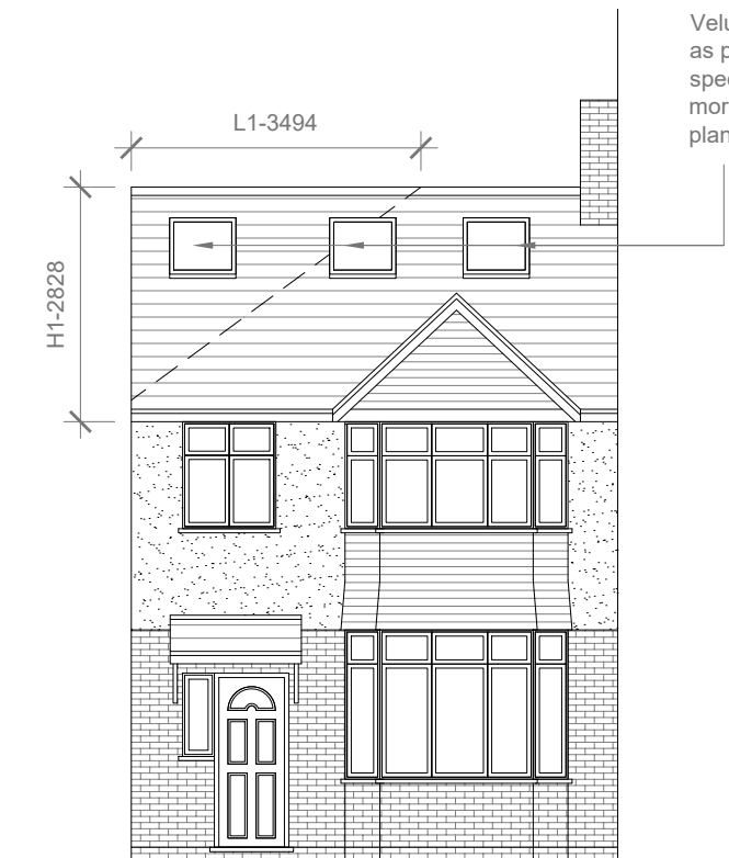
Proposed Front Elevation Scale 1:100
