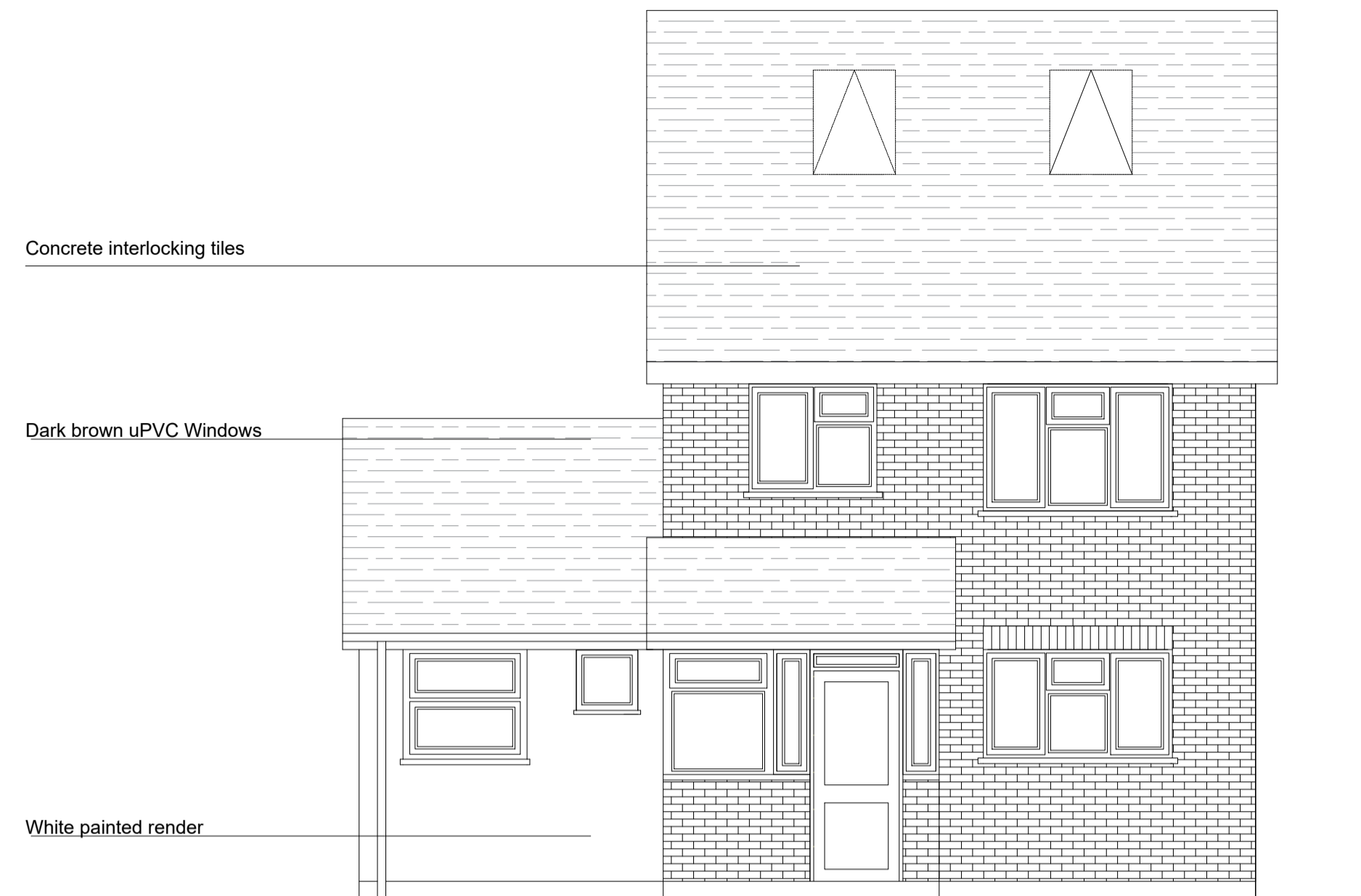
EXISTING FRONT ELEVATION A
