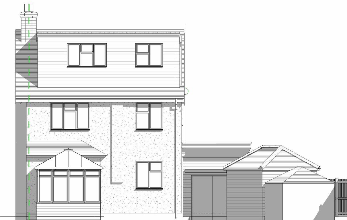
3 Existing Rear Elevation 1 : 100
