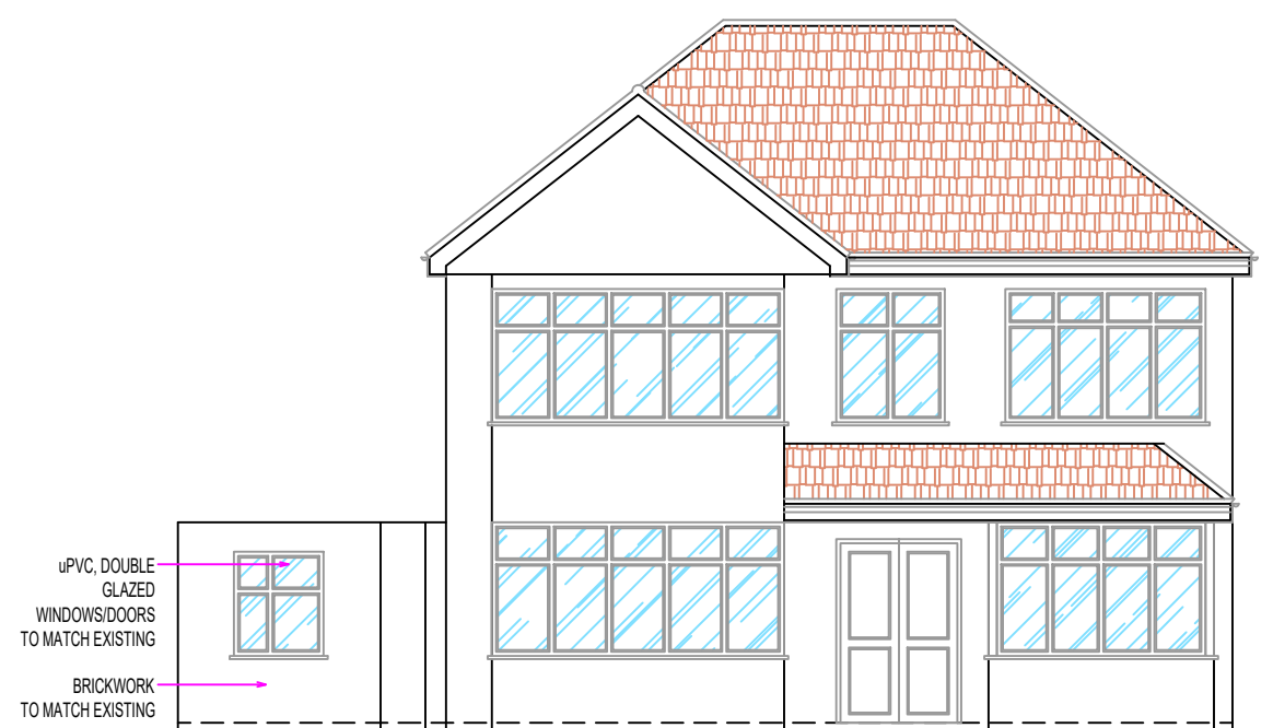
PROPOSED FRONT ELEVATION SCALE 1:100@A1
