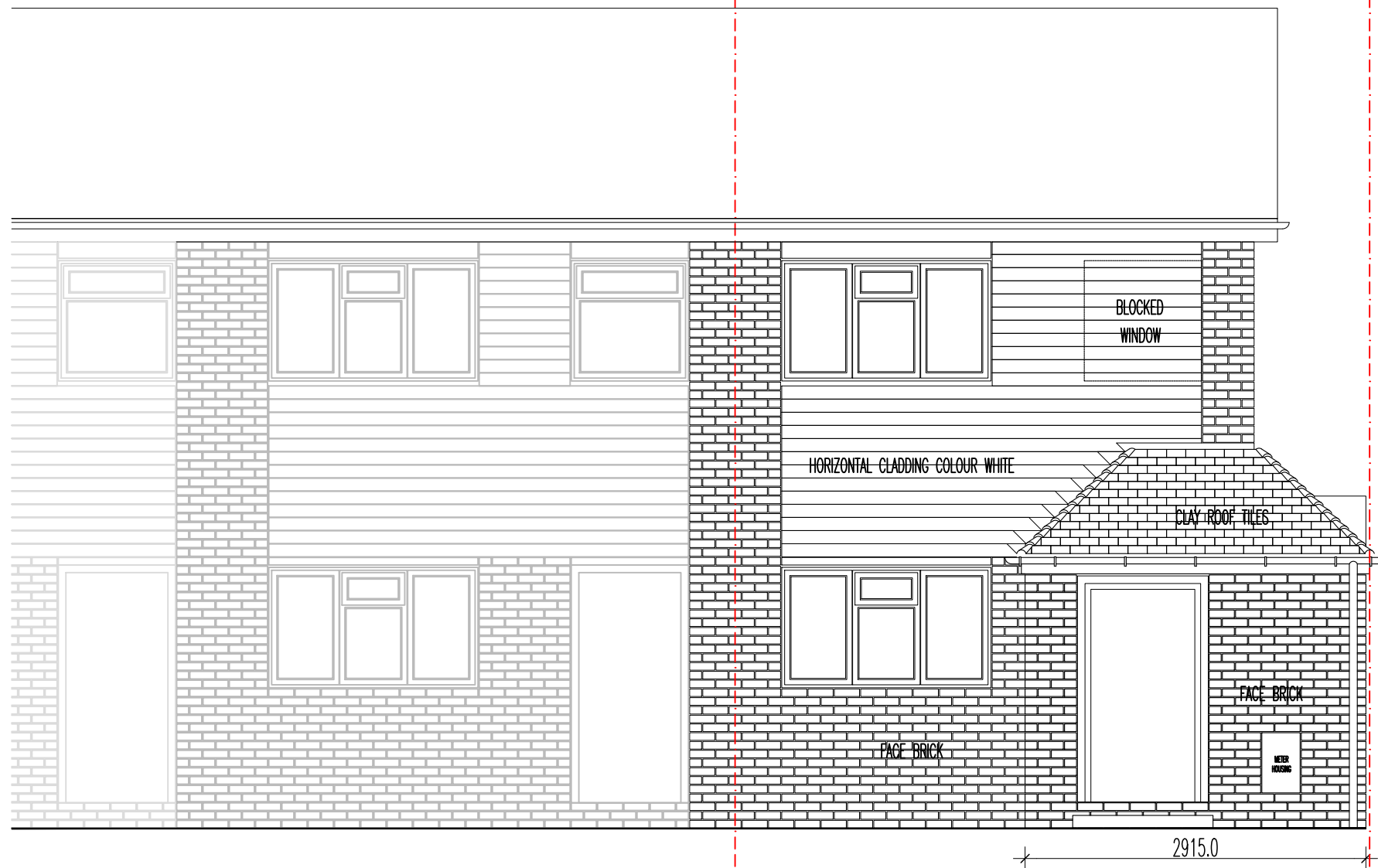
FRONT ELEVATION AS BUILT
