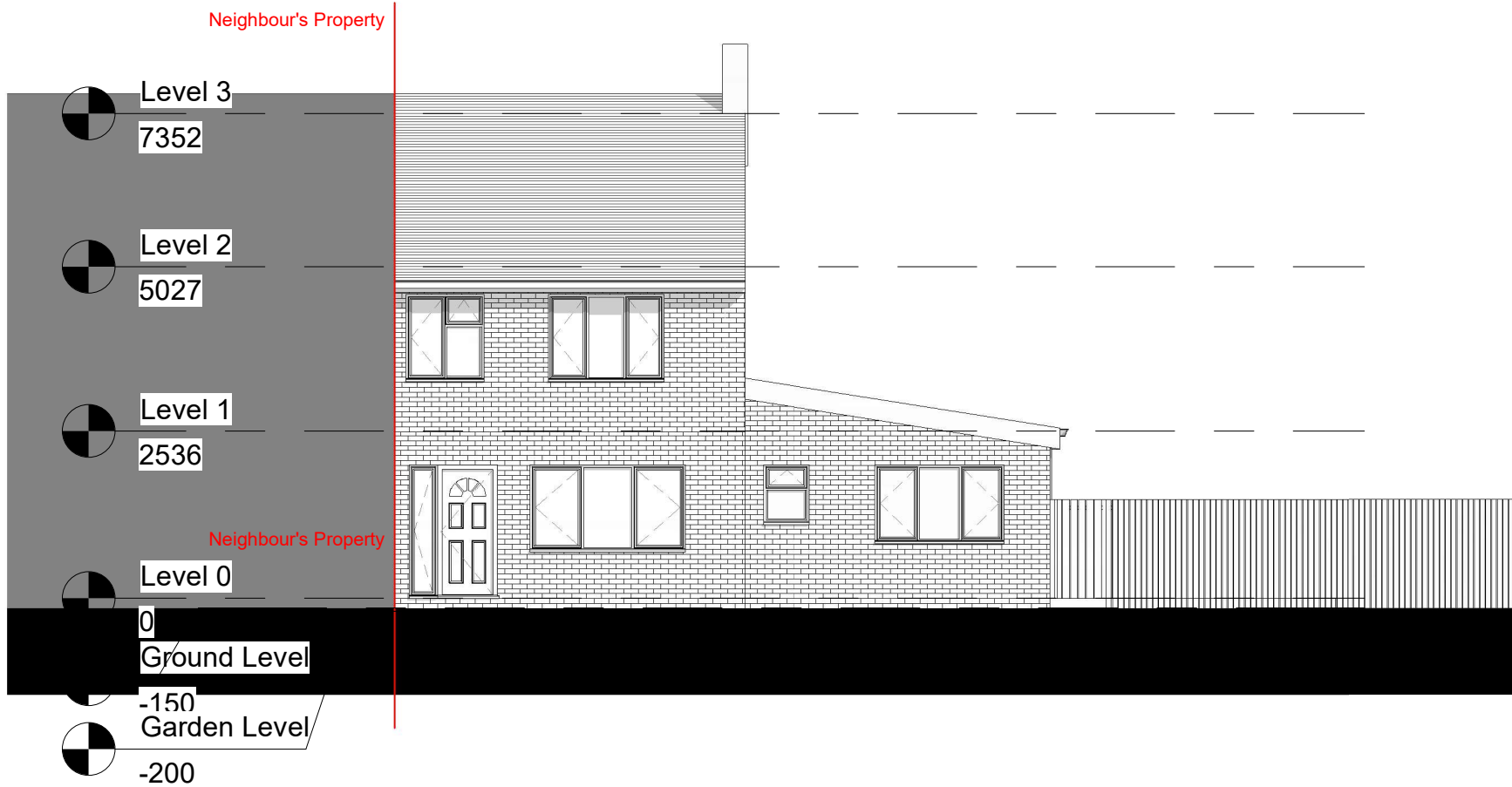
2 Front Elevation Proposed 1 : 100
