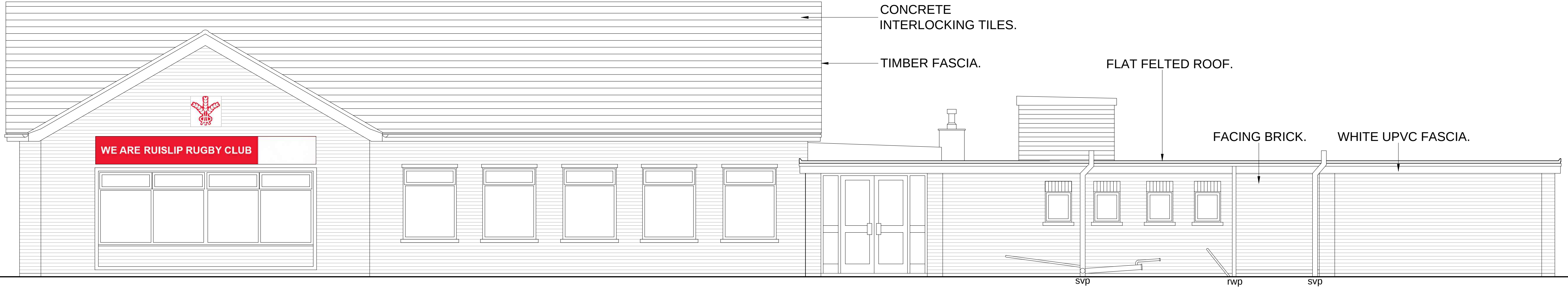
EXISTING FRONT ELEVATION (EAST FACING)
