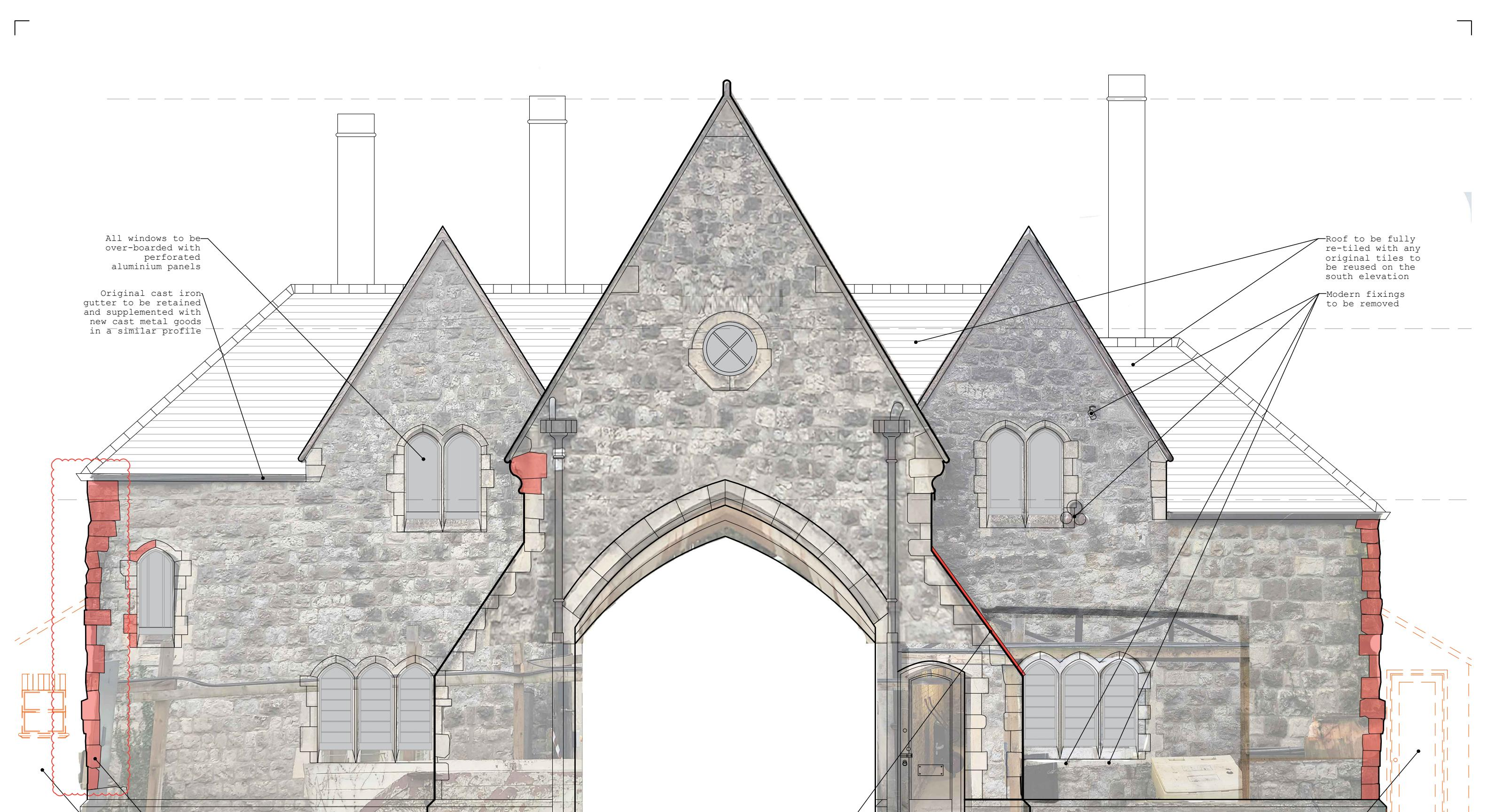
stone quoins have been lost where modern extension was added. to be repaired and new stones inserted to ensure a clean corner is reinstated.
