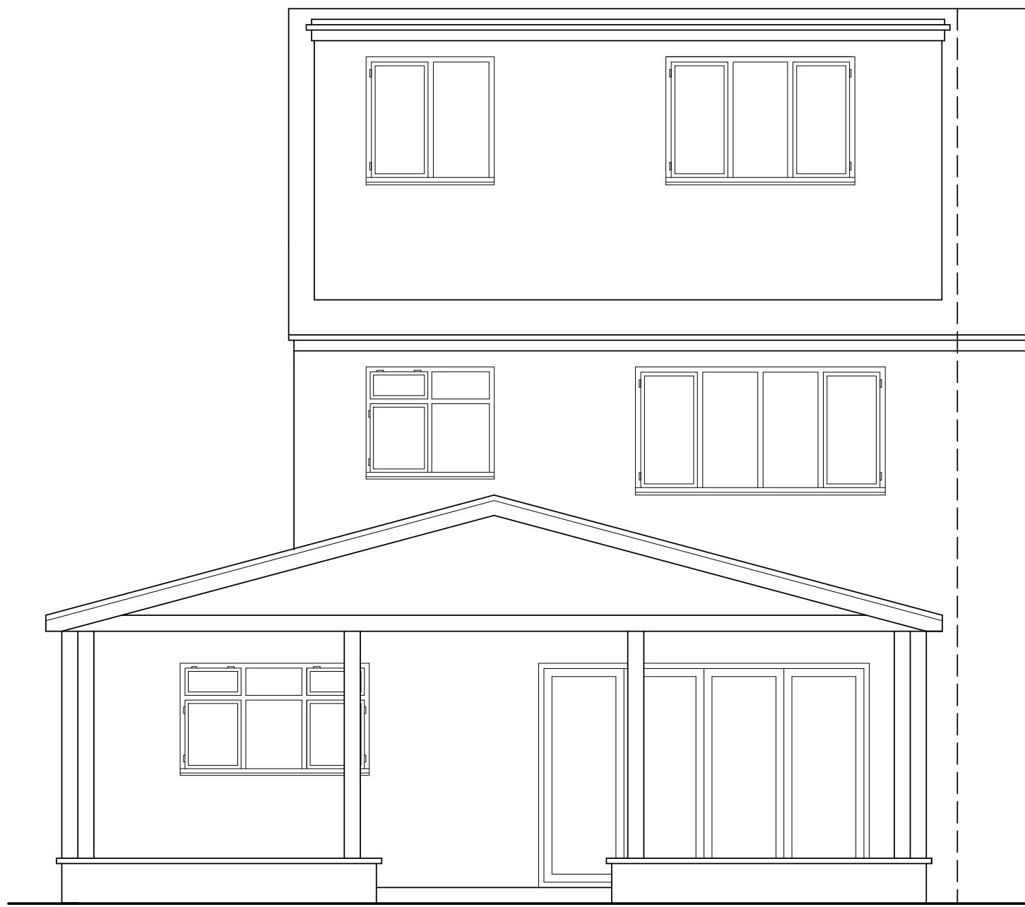
EXISTING REAR ELEVATION - 1:50
