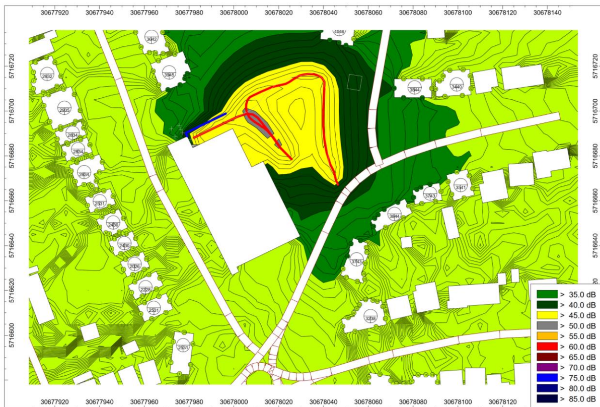
Figure 6: Day-time noise map of delivery vehicle arrival ( L_{Aeq,1hour} , 4.5 metre height)
