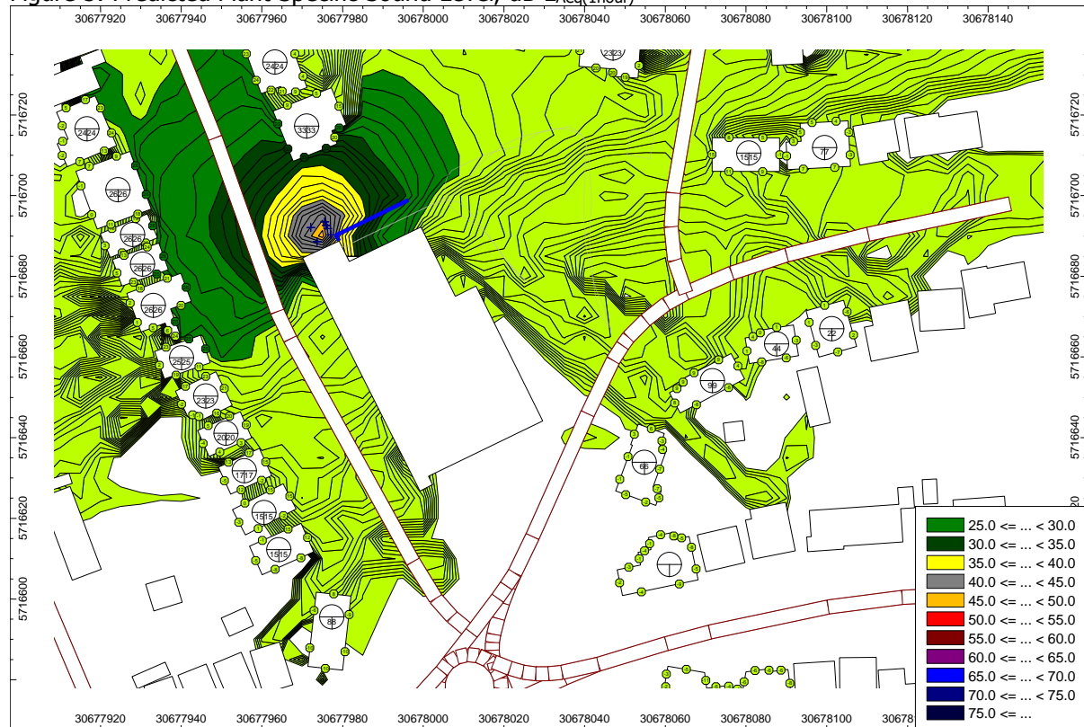
Figure 5: Predicted Plant Specific Sound Level, dB LAeq(1hour)
