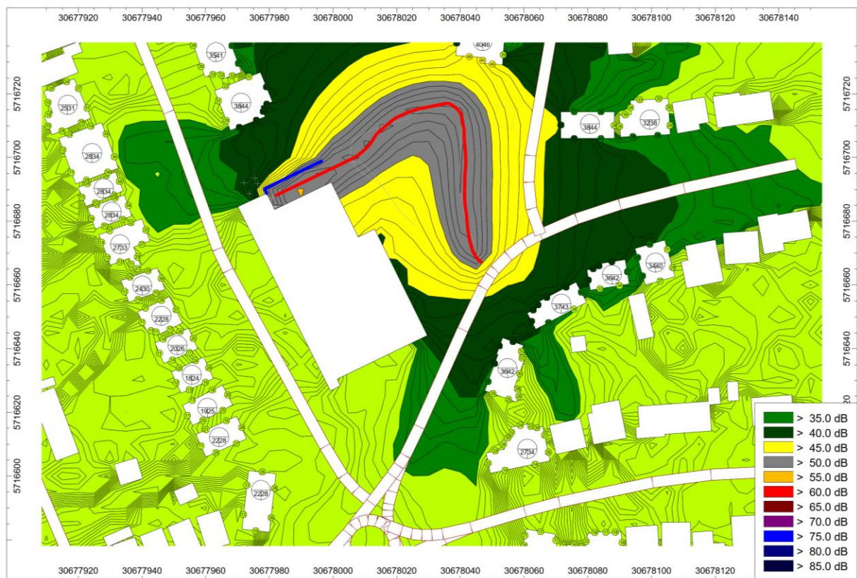
Figure 8: Day-time noise map of delivery vehicle departure ( L_{Aeq,1\text{ hour}} , 4.5 metre height)
