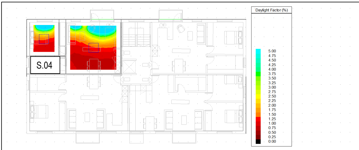
Figure 12: FlucsDL Daylight Factor Levels – Second Floor
