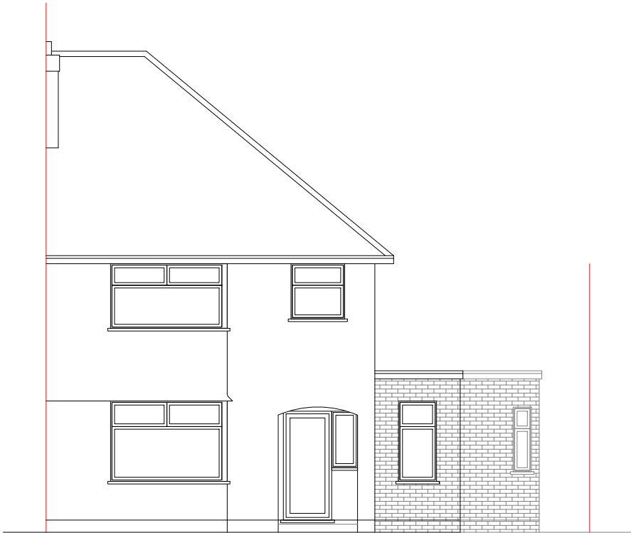
Proposed Front Elevation Scale 1:100
