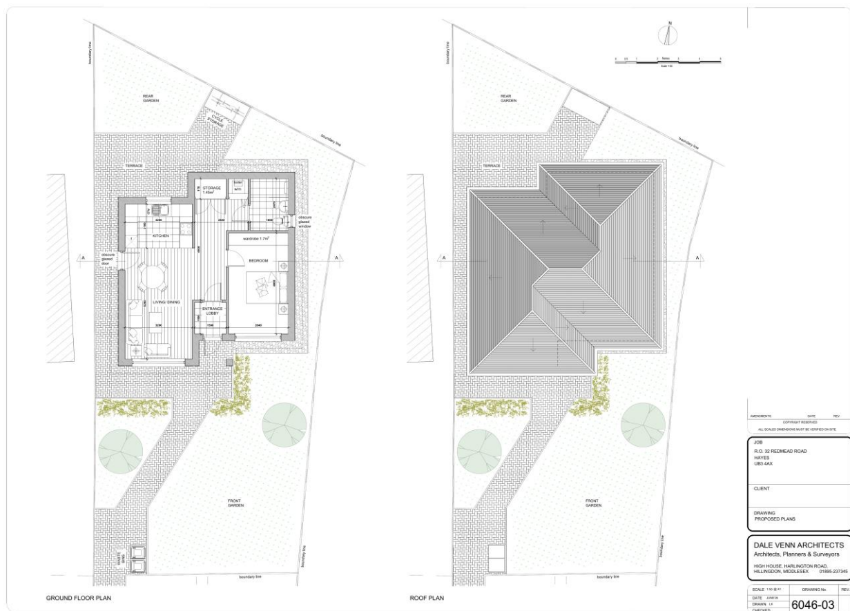
Proposed ground floor and roof plans - drawing 6046-03, showing 1.45 sq.m dedicated storage and 1.7 sq.m built-in wardrobe storage.
