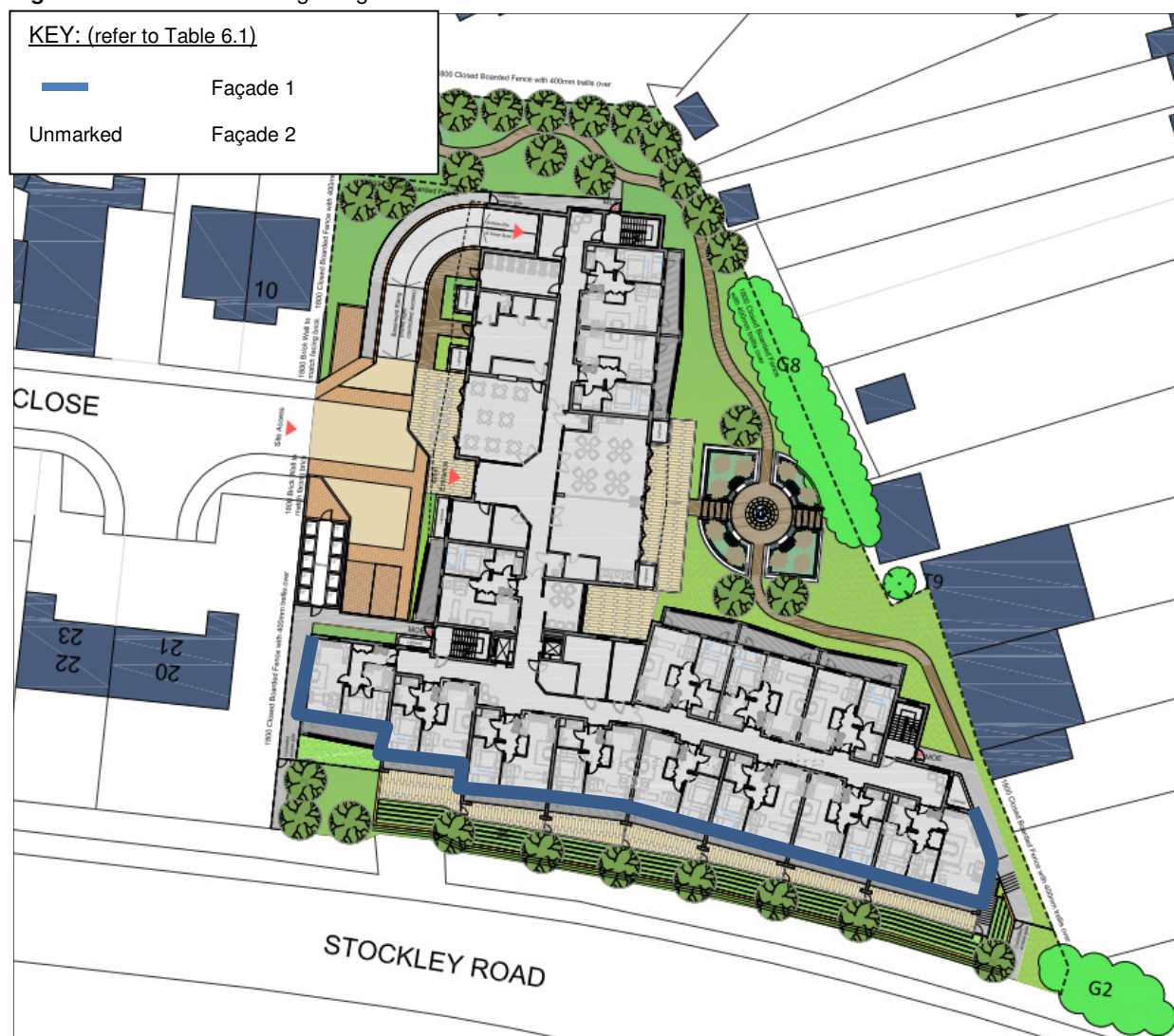
Figure B.1: Recommended glazing & ventilation Locations.
