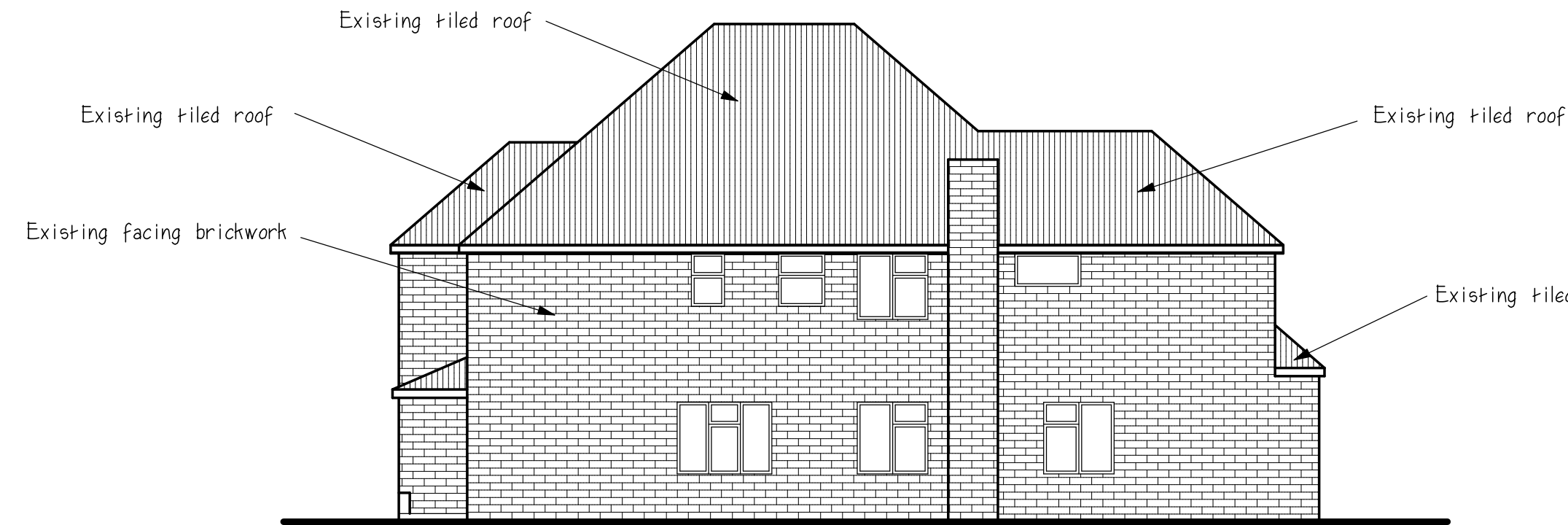
Existing side elevation
