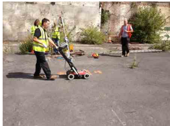
Ground Penetrating Radar surveying
