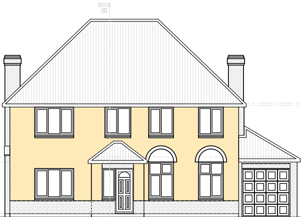
EXISTING FRONT ELEVATION
