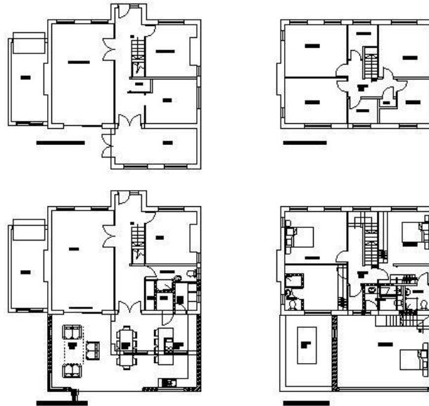
5.4 The first floor comprises of merging existing bedroom 1 and 2 to one single room which accommodates bedroom with en-suite and walking wardrobe. The other existing front room has been enlarged and accommodation en-suite. The new rear extension will accommodate a large Master Bedroom on two floors. The first floor would be used as bedroom and the second floor (area in part of the loft) would be used for dressing and entertainment area.
