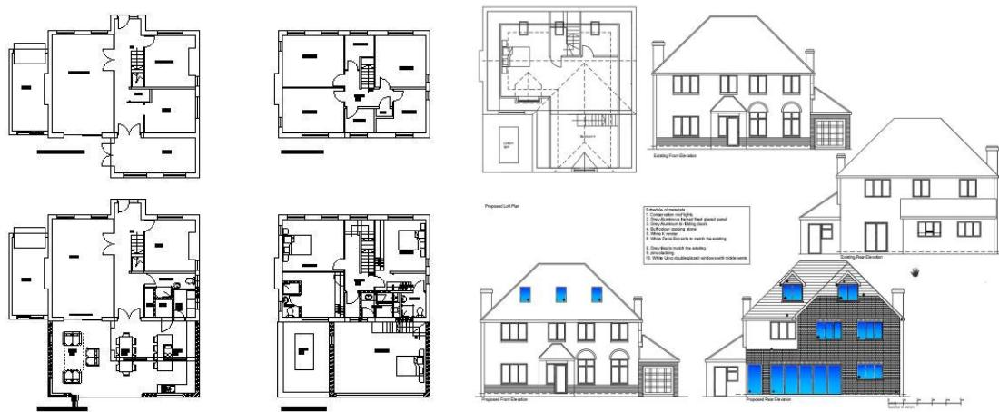
5.5 The existing front shower room would be taken out and replaced with a new staircase leading to the loft bedroom 4. The bedroom 4 would comprise of en-suite and study area.
