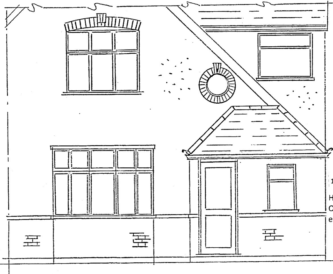
Proposed Front Elevation 900mm x 2100mm door frame size Allow for low threshold sill
