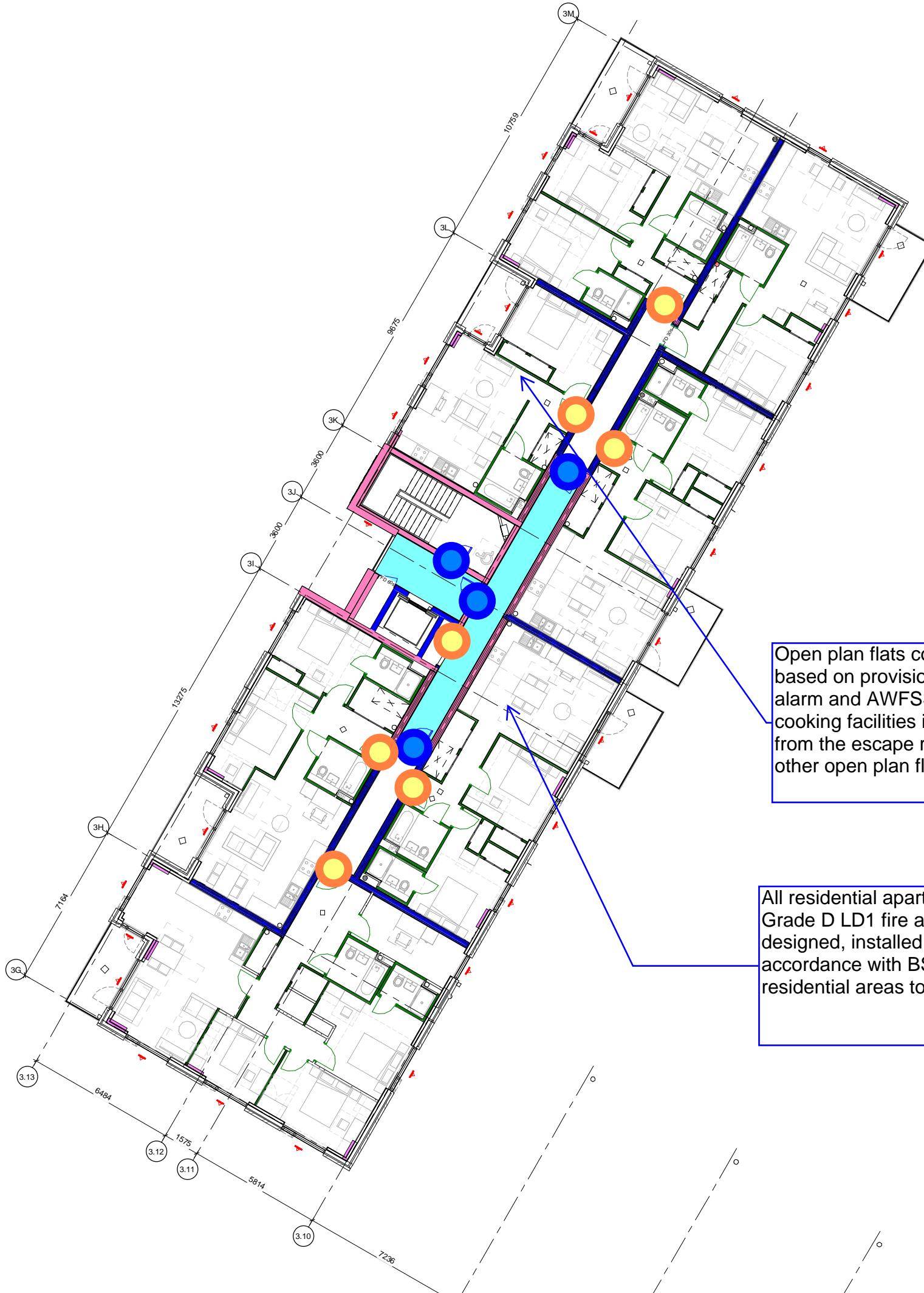
Open plan flats considered acceptable based on provision of Grade D LD1 fire alarm and AWFSS in the flat, and the cooking facilities is located at least 1.8m from the escape route. This applies to all other open plan flats.
