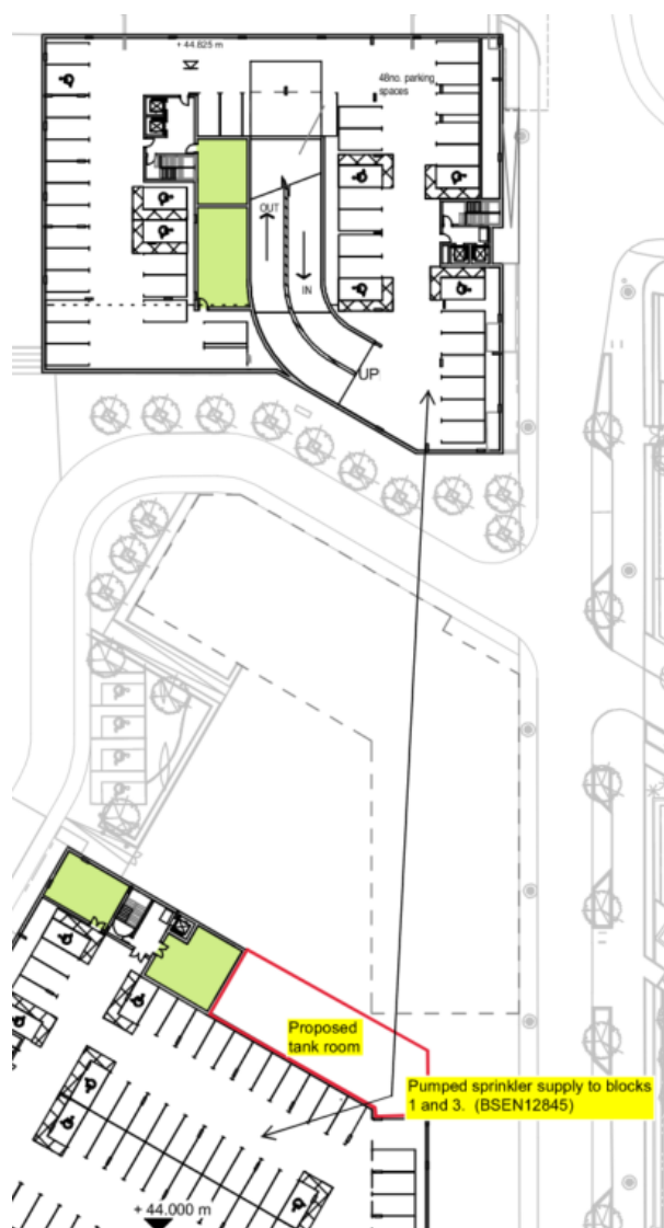
Figure 13 - Water delivery to sprinkler system in Block 1 building
