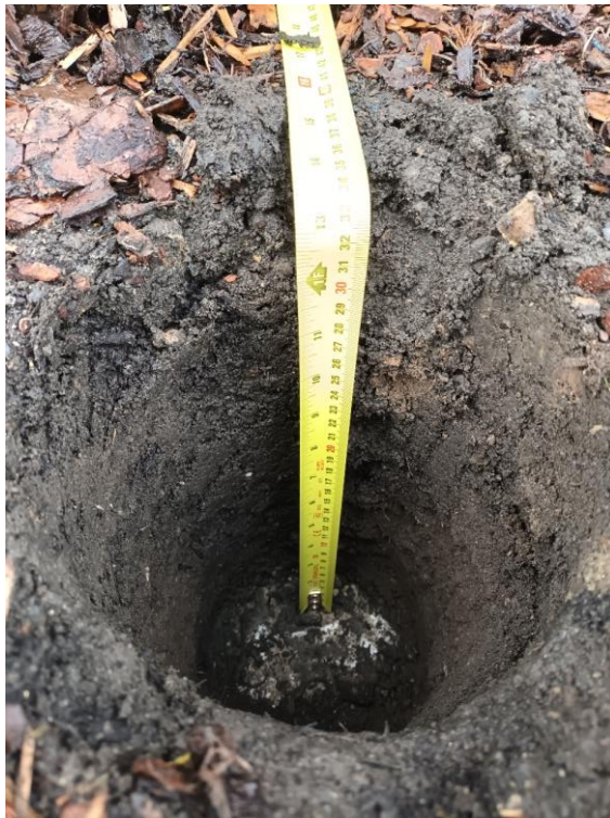
Showing the thickness of the topsoil cover and the presence of the white membrane at the base.
