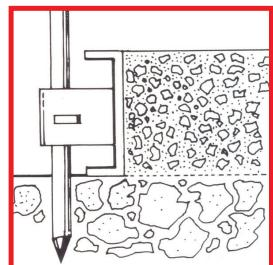
Roadforms provide a simple, robust, accurately aligned edge formwork for use when constructing ground slabs, roadways, pathways and foundations up to 300mm. Made of strong square section steel and using a series of ground stakes to secure in place. Roadforms create a smooth uniform finish to any poured concrete slab. Each Roadform is tongued to allow continuous runs.
