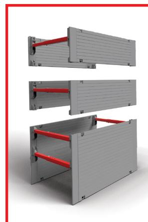
The Mini Trench Box can be used in trenches up to 4000mm deep with widths from 610mm to 3200mm, which can be altered using telescopic struts. Up to two extension boxes can be added on top of the mini Trench Box to achieve additional depth.
