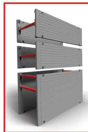
The Standard Trench Box is used to provide a safe working area below ground and ensure that the side walls of an excavation are continually supported. Standard Trench Boxes can be used in conjunction with other boxes, including Manhole Boxes. They are quick and easy to install.
