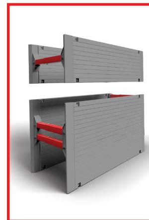
The Drag Box acts as a shield to protect users in self-supporting soil. It is designed to withstand up to 25kN/m<sup>2</sup>. Installation requires the 'Excavate and Drag' technique, the box is placed in a pre-dug trench and moved after each instalment of pipe.
