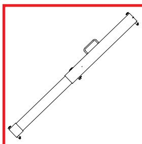
Our Aluminium Waler End Bearer system has been developed to be used with a wide range of Aluminium Waler Rails to provide lightweight support to non-battered ends of trenches. To be used in conjunction with Trench Sheets/existing Waler systems, this product offers a safe and efficient replacement to less suitable methods, such as timber or road plates, by retaining backfill, preventing accidental dislodgement of loose material and also a barrier to prevent unauthorised access to the excavation
