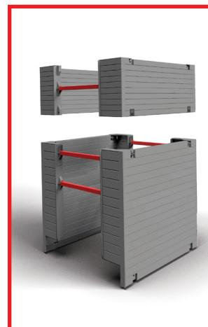
The Backhoe Manhole Box is a four-sided excavation box which provides a safe working area below ground. The Backhoe Manhole Box can sustain earth pressures of 20kN/m<sup>2</sup>. Users should check that the excavation will impose no greater pressures than this.
