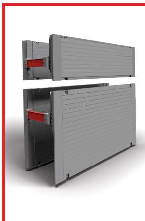
The Maxi Drag Box is ideal for use with long pipe runs, the size increases productivity allowing for a faster installation time. The Maxi Drag Box can be installed using the 'Excavate and Drag' technique. The box is placed in a pre-dug trench and pulled along the trench as each section of pipe laying is completed.
