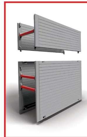
The Backhoe Trench Box is a robust piece of equipment, which acts as a safety shield to provide a safe working area below ground level. For use when working on excavations and pipe laying operations. The Backhoe Trench Box can sustain working earth pressures of up to 20kN/m<sup>2</sup>, users should check that the excavation will not impose greater pressures than this.
