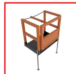
Manufactured from mild steel with a powder coated finish. Specially designed for use on all types of box and sheeted excavations. Cantilevered platform enables safe side-entry onto ladder. Standard pole ladder fits directly onto the unit and is locked in place with two ladder clamps. Adjustable clamps fit directly onto a Trench Box or sheets (two sheet clamps and two box clamps supplied with platform). Adjustable front legs for ease of levelling. Collapsible sides and gate for ease of storage.
