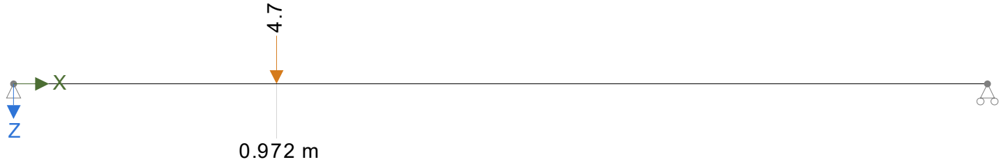
Permanent - Loading (kN)
