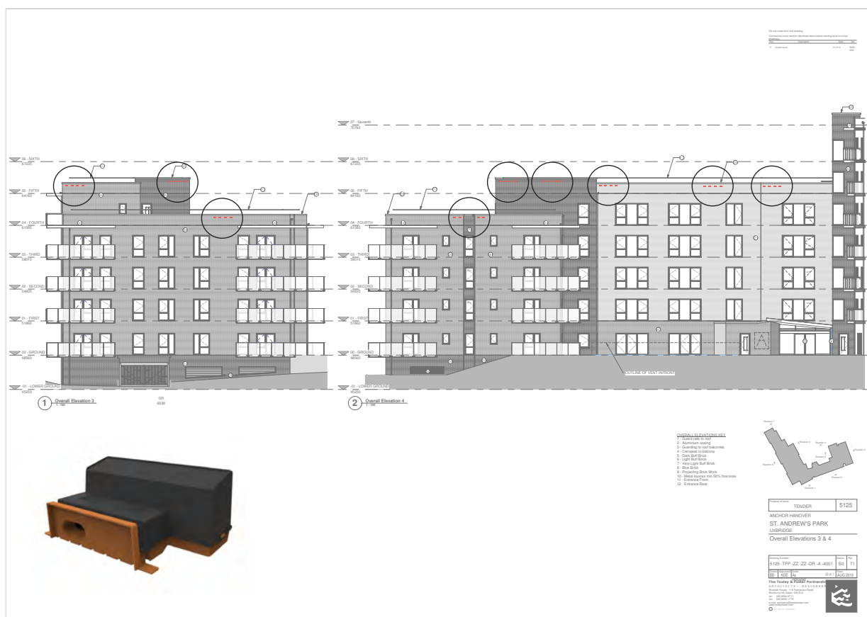
Location of 36 no. Manthorpe Swift Bricks (9 groups of four bricks)
