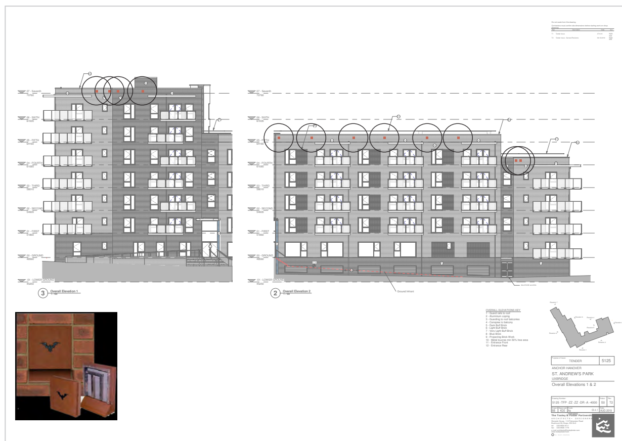
Location of 12 no. Ibstock Enclosed Type C Large bat boxes
