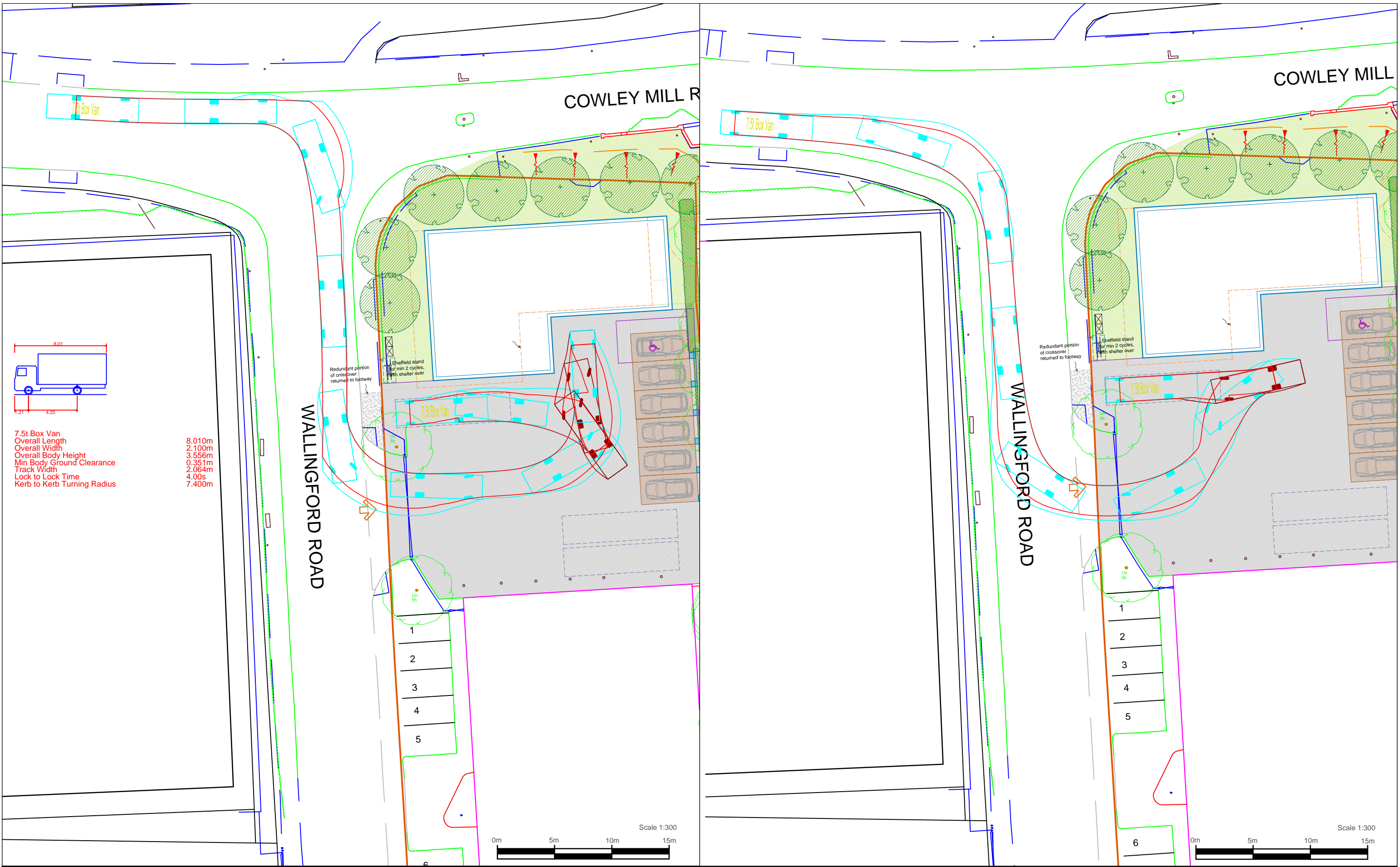
P3006: GRANVILLE HOUSE, WALLINGFORD ROAD, LONDON, UB8 Figure SK3. Swept Path Analysis; 7.5t Box Van Enter Site & Reverse to Lorry Bay (L), Exit Site Forwards (R)
