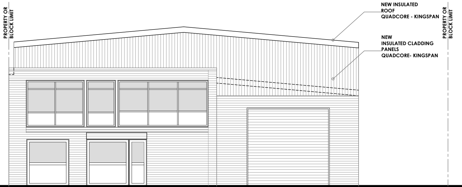
PROPOSED FRONT ELEVATION SCALE 1/100
