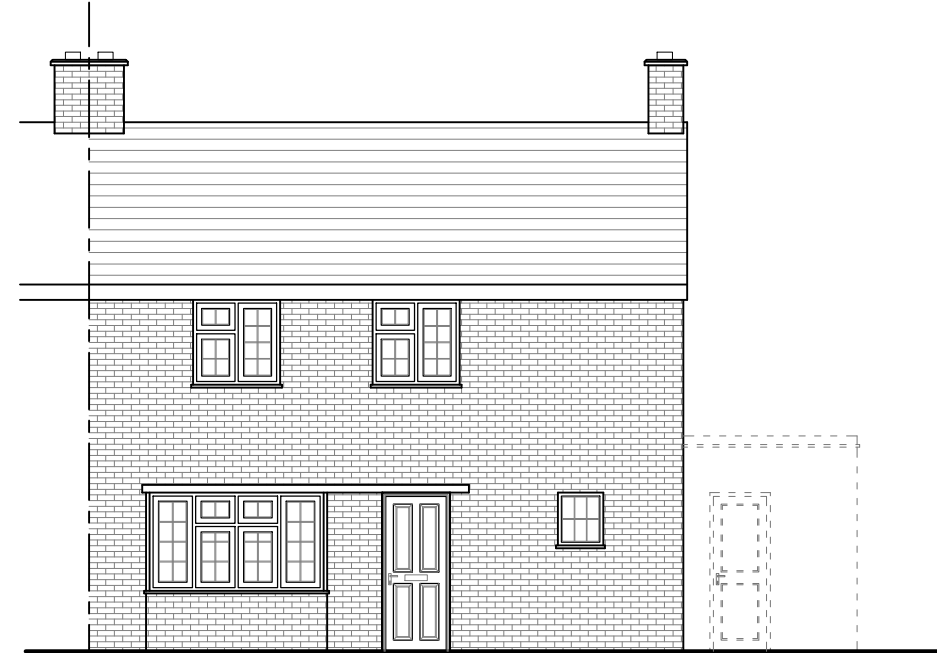
PROPOSED FRONT ELEVATION SCALE= 1:100
