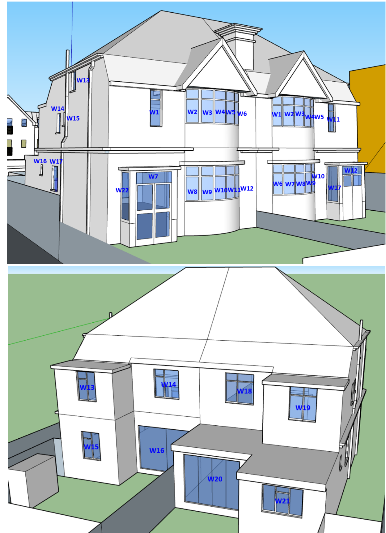
Figure 4.5: Assessed Windows at the Adjacent 551 and 553 Uxbridge Road
