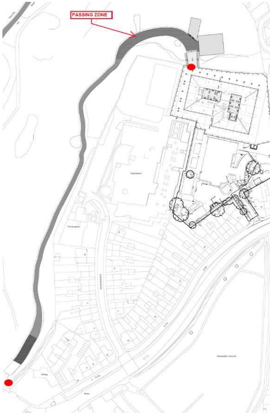
Figure 16 Haul road plan showing gate team locations and passing zone
