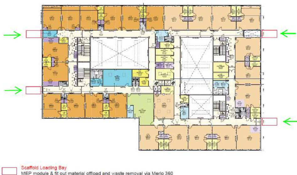
Figure 36 Offloading and distribution to Level 1 and roof
