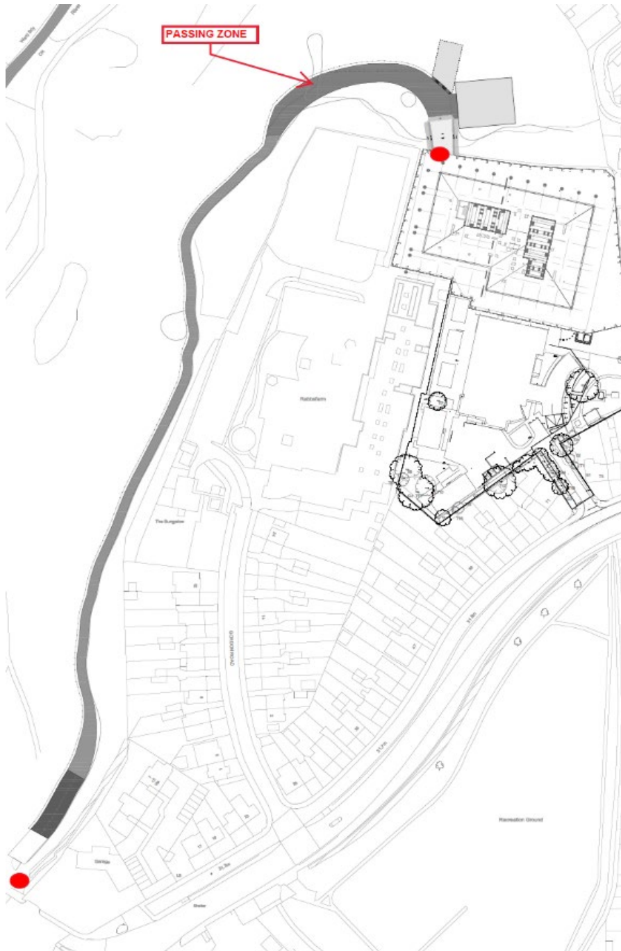
Figure 16 Haul road plan showing gate team locations and passing zone
