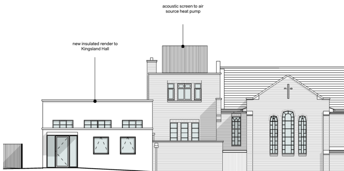
Figure 6 Elevation showing the screen
