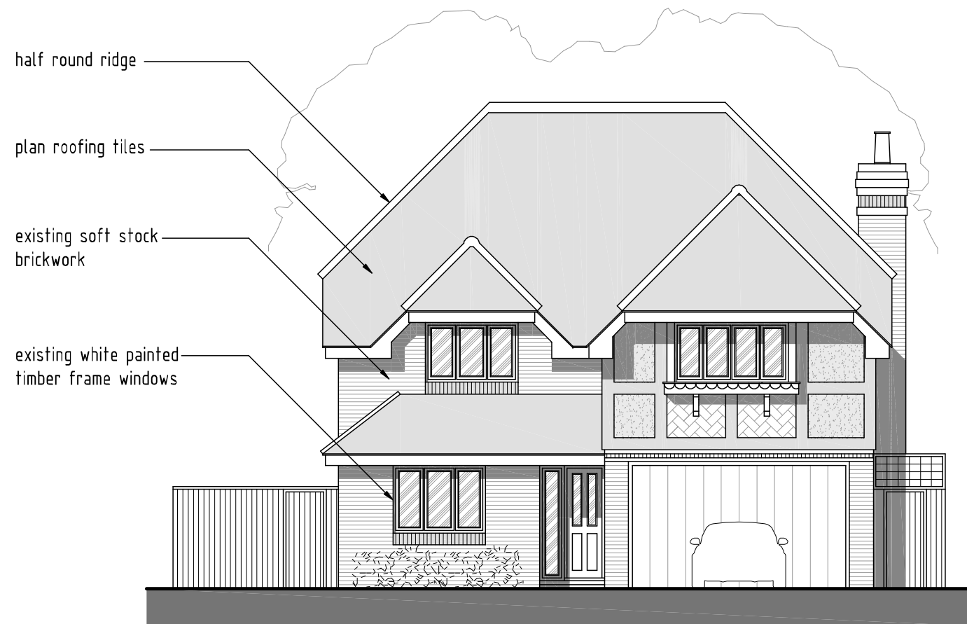
EXISTING FRONT ELEVATION - 1:100
