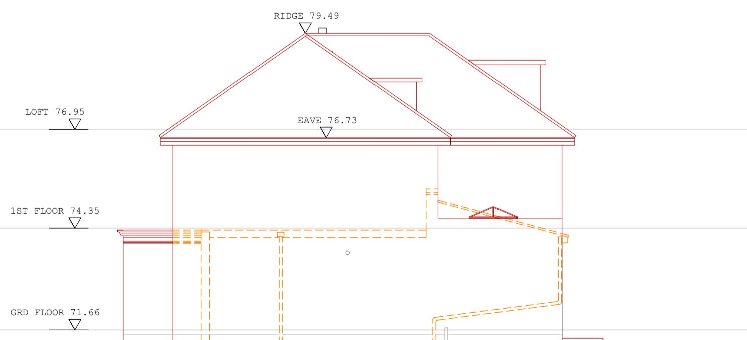
FLANK ELEVATION (RESTRICTED VIEW) DATUM LEVEL 70.00m
