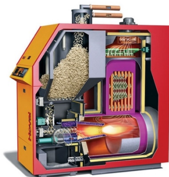
Figure 4: Biomass Boiler diagram
