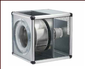
GB.. T120: The motor which is located outside of the air flow is separated from the impeller through a temperature insulated partition panel. The motor-impeller-unit is removable without disassembly of the ducting.
