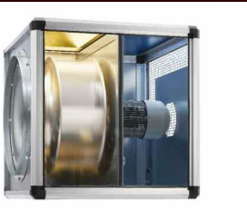
GB.. T120: The motor which is located outside of the air flow is separated from the impeller through a temperature insulated partition panel. The motor-impeller-unit is removable without disassembly of the ducting.
