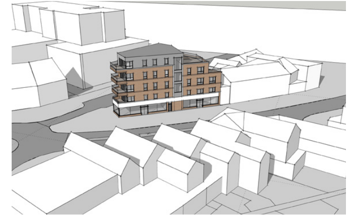
Image 3 Proposed Building | 5-storey building with metal clad top storey and feature balconies to front. (Pre-planning design)
