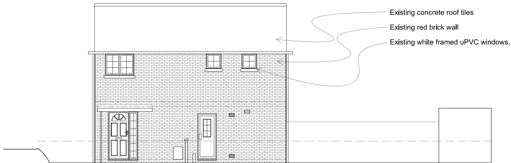
EXISTING EAST ELEVATION
