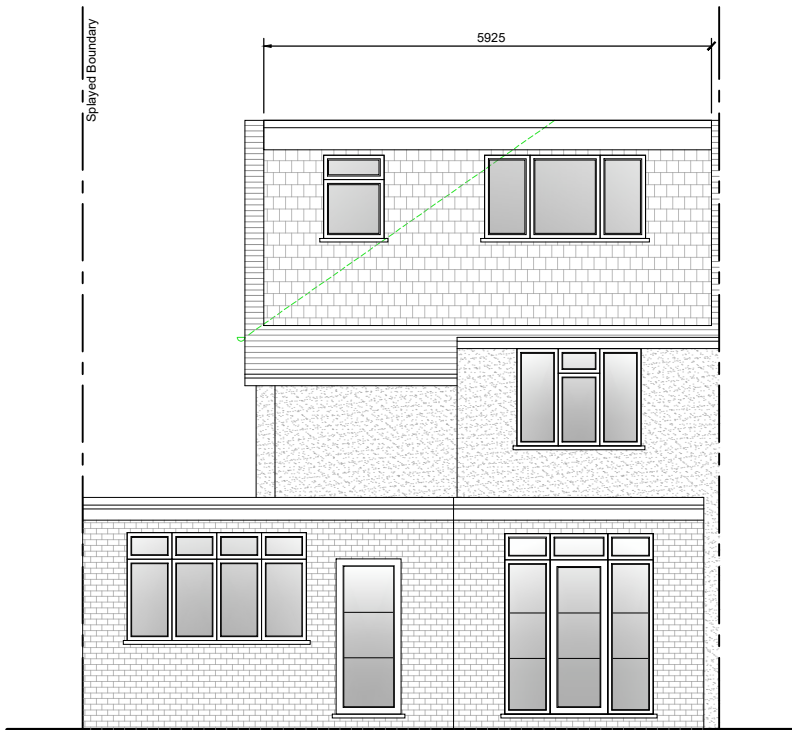
Proposed Rear Elevation Scale 1:100
