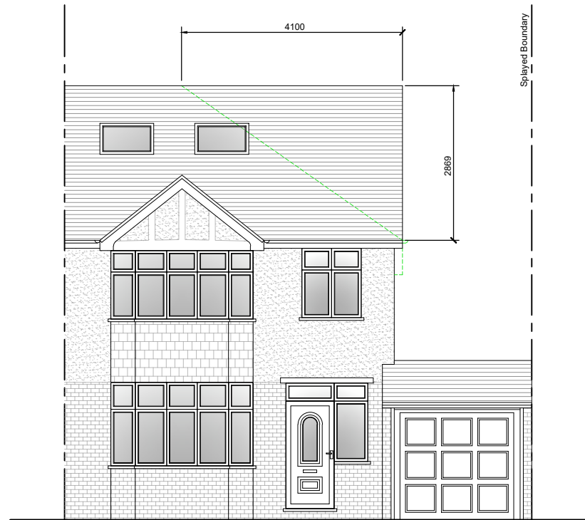
Proposed Front Elevation Scale 1:100
